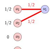
$$egin{aligned} \max \sum_{e \in \mathcal{E}} x_e \ & \sum_{e \in \delta(v)} x_e \leq 1 \quad orall v \in \mathit{U} \cup \mathit{V} \ & x_e \geq 0 \quad orall e \in \mathit{E} \end{aligned}$$
